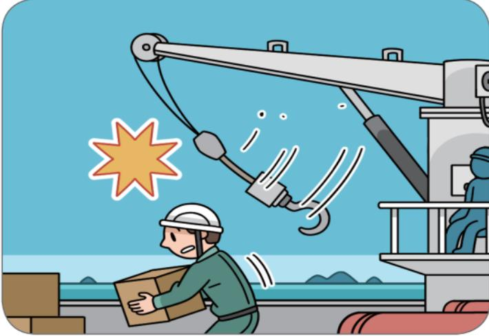
While adjusting the position of the hook of a crane for loading food, the deckhand signaled to lower the crane boom but the boatswain, who was operating the crane, misunderstood it as a signal to lift the boom and moved the boom to the left side. It lightly struck a worker who was preparing the loading on land on the head. If it had struck with greater force, it could have been a marine incident that resulted in a serious head injury.
