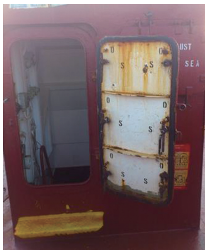
Figure 4.2 The weather-tight door on the fore-castle deck SOURCE Investigation report(HKSAR)
