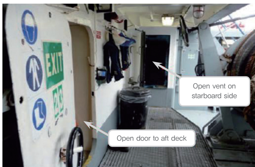
Figure 13.3 The door leading to the after deck on the tug(sister ship) SOURCE Investigation report(The Dutch Safety Board)
