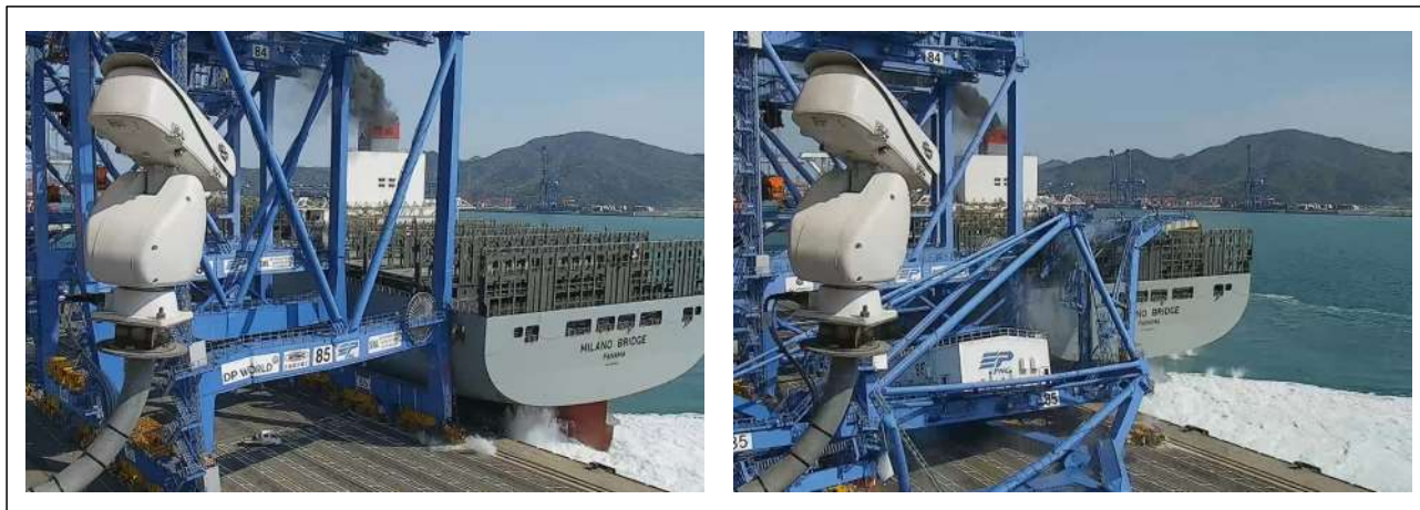
<Figure 23> Collision between Milano Bridge and the gantry crane (CCTV)
