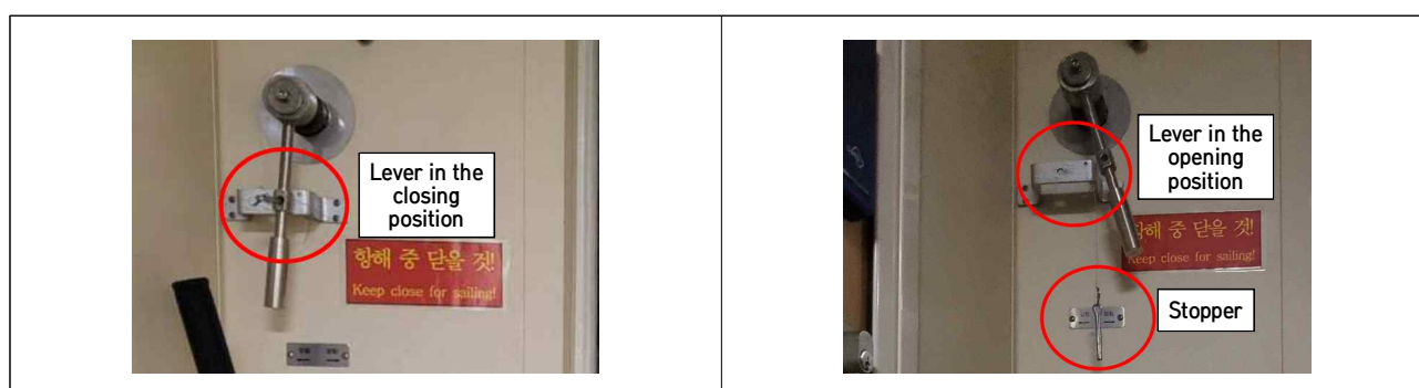
<Figure 14> Closed control lever in the corridor (left) and opened lever (right)
