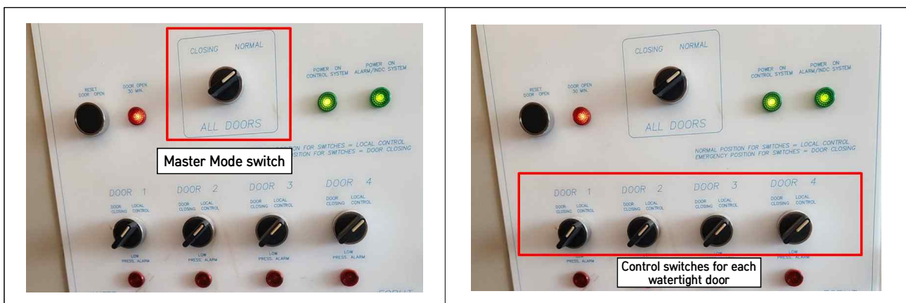
<Figure 18> Control console for watertight doors onboard Onnuri
