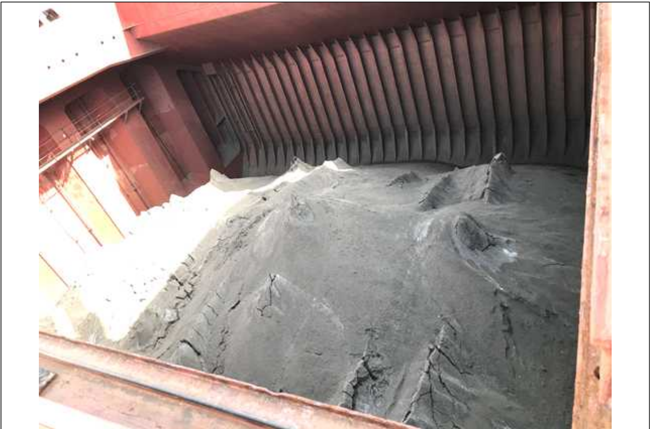
<Figure 10> Appearance of the cargo being loaded into the cargo hold at the time of the accident
