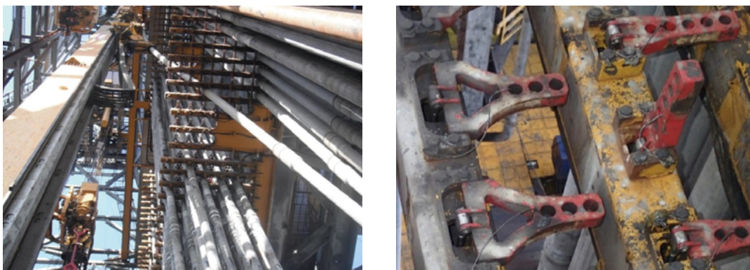
Figure 8.2 Drill Pipes · Latches SOURCES Investigation Report (LIBERIA MARITIME AUTHORITY)
