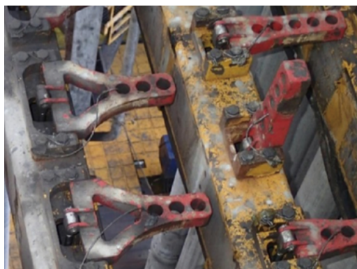
Figure 8.2 Drill Pipes · Latches 출처 Investigation Report (LIBERIA MARITIME AUTHORITY)
